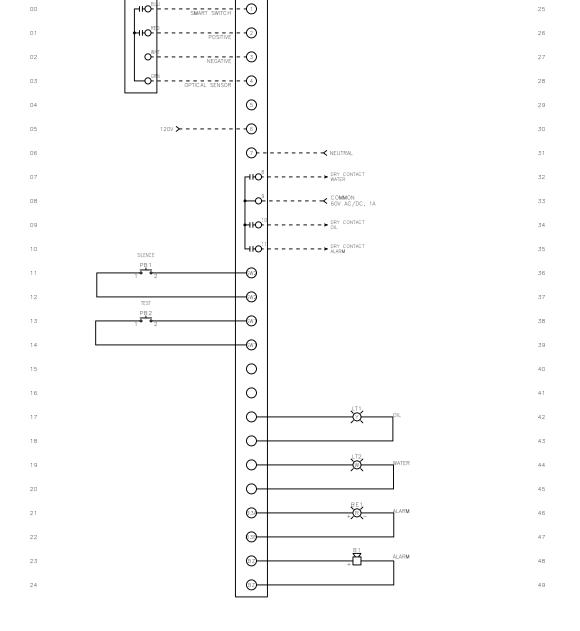
DASHED LINE INDICATES FIELD WIRING.
